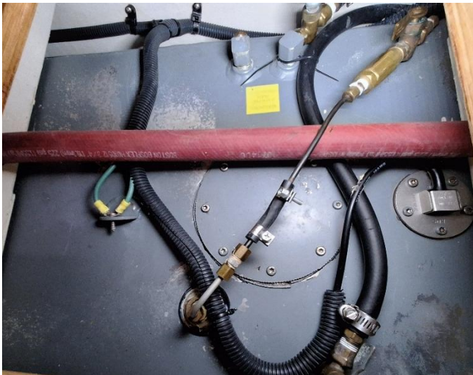
Picture 12: Diesel fuel tank with shut-off valve and fuel vent (top right).
