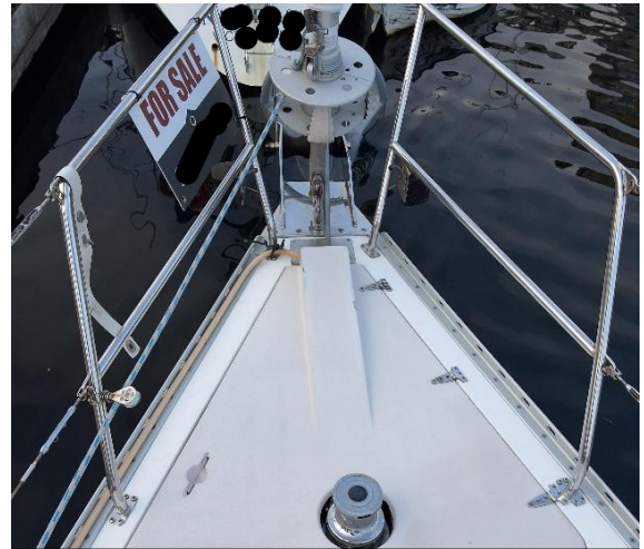
Picture 7: Anchor locker bow hatch with windlass and headsail Furler.
