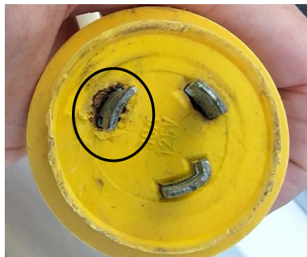
Picture 13: Shore Power cable plug with damaged terminal.
