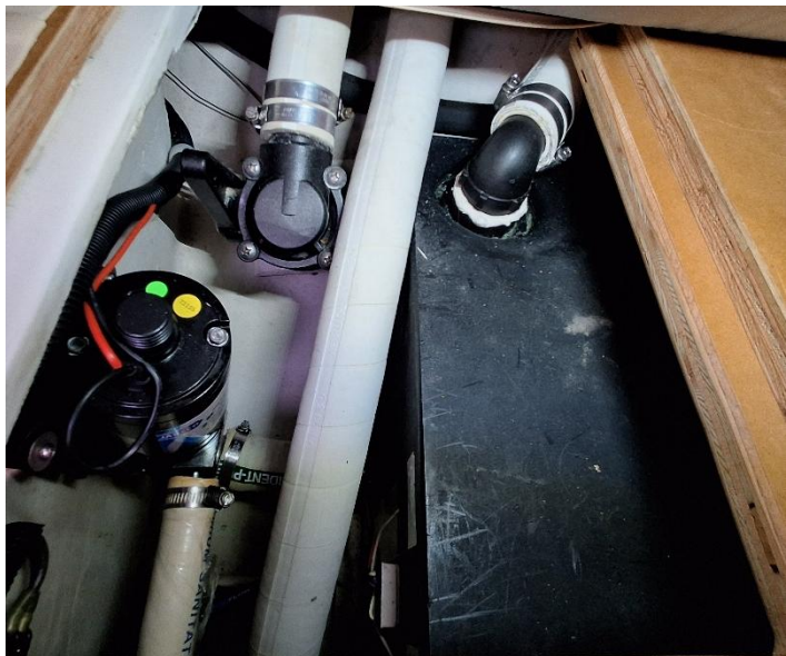
Picture 24: Black sewage tank with JABSCO macerator pump located port side mid-ship.
