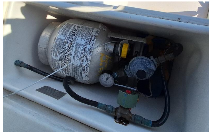
Picture 23: Propane cylinder within a dedicated propane locker located at the starboard transom.
