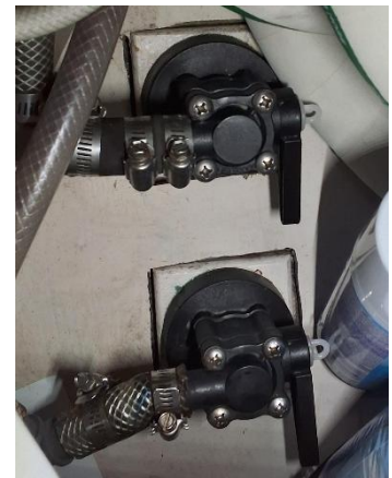
Picture 5: Two MARELON through-hull fittings; top for starboard side shower sump and lower for starboard head sink drain.
