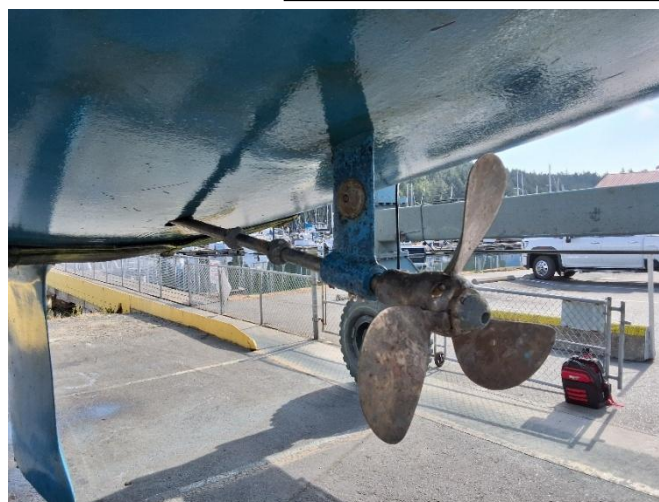
Picture 10: Folding propeller, strut, anodes and shaft.
