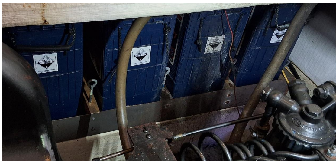
Picture 36: Port side battery bank. Four of six batteries visible. Noticed battery fluid run-off on the side of the batteries. Several terminals were seen corroded.
