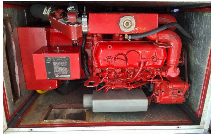
Picture 26: WESTERBEKE marine diesel generator within insulated case box. Located aft in engine room.
