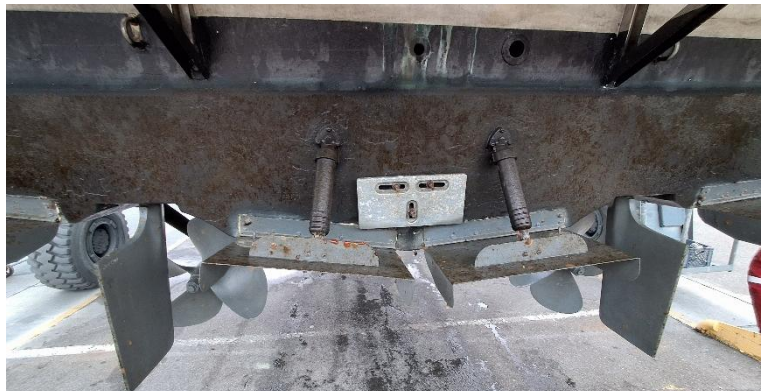
Picture 28: Stern view of running gear including anode, trim tabs, rudders and propellers.
