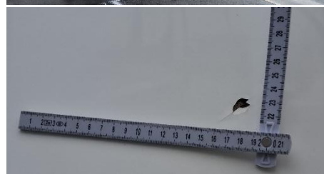
Picture 5 and 6: Starboard bow impact affecting gelcoat.
