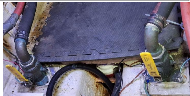
Picture 14: Main engines saltwater intake for cooling system. Double clamped and tested by hand only.
