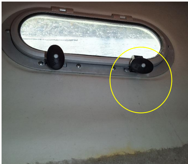
Picture 9 (Left): Inside view of port side bow porthole. Rust stain and corrosion visible on aluminum fasteners. Same condition on starboard side portholes. (not pictured)
