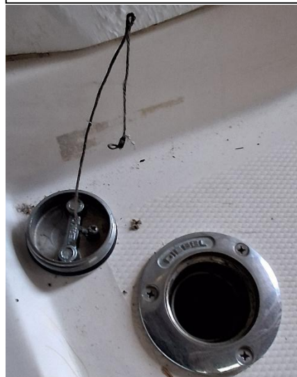
Picture 30: Port side fuel fill cap not permanently attached.
