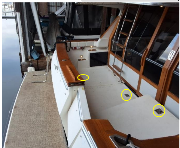
Picture 21: Aft cockpit access hatches (3) with damaged handles.
