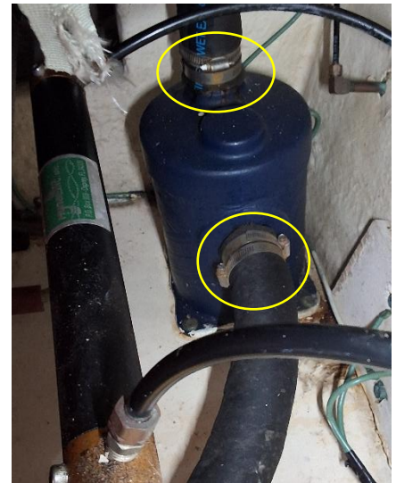
Picture 27: Generator's exhaust hose clamps showing surface rust. Also visible is the HYNAUTIC steering cylinder.
