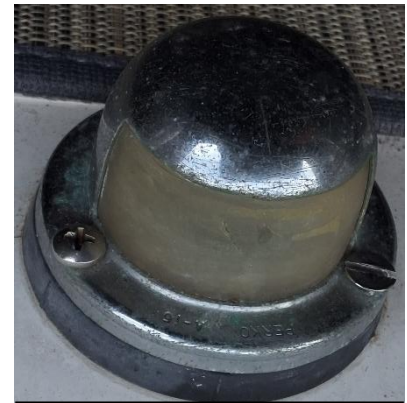
Picture 39: Stern light lens crazed and cracked.
