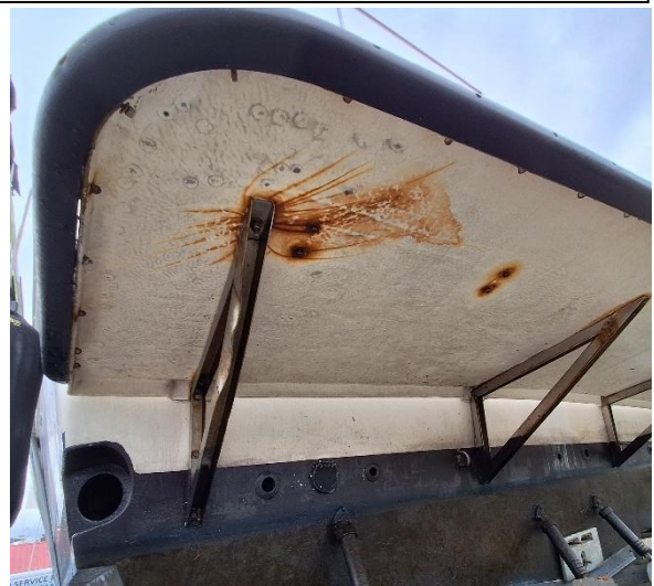
Picture 8: Under view of swim grid showing rusty attachment bolts for re-boarding ladder. Also showing FRP stress cracks.
