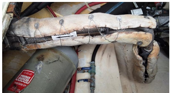
Picture 44: Port aft diesel heater with damaged exhaust insulation and rusty clamps.
