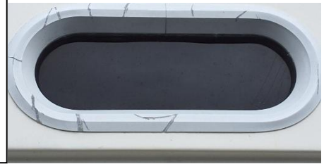
Picture 10 & 11 (Right): Starboard side portholes frame at the bow, outside view. Showing scratches and impact damage around the frame's perimeter.
