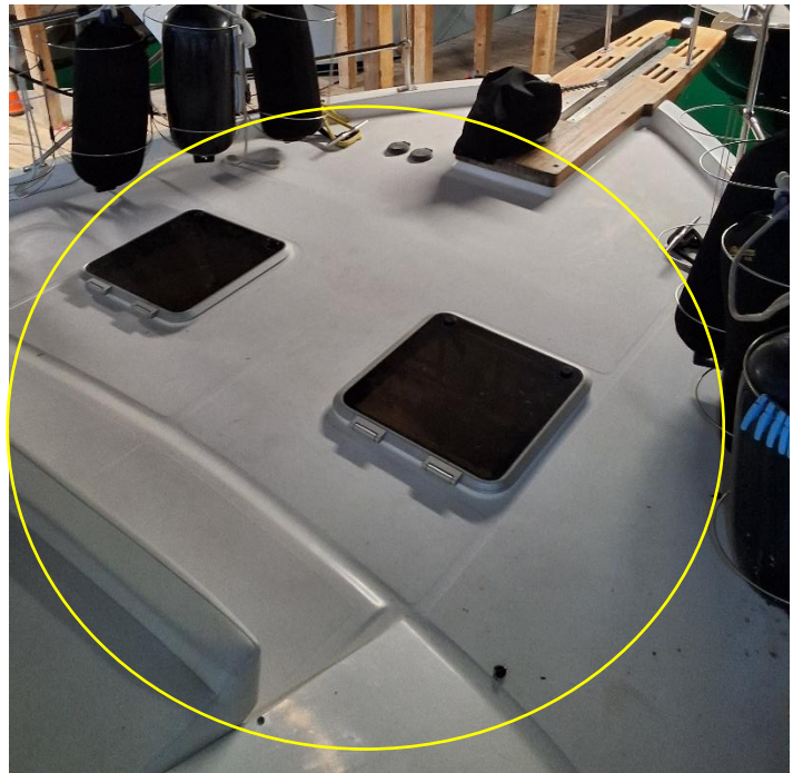
Picture 7: Bow deck view showing elevated moisture and soft spot.
