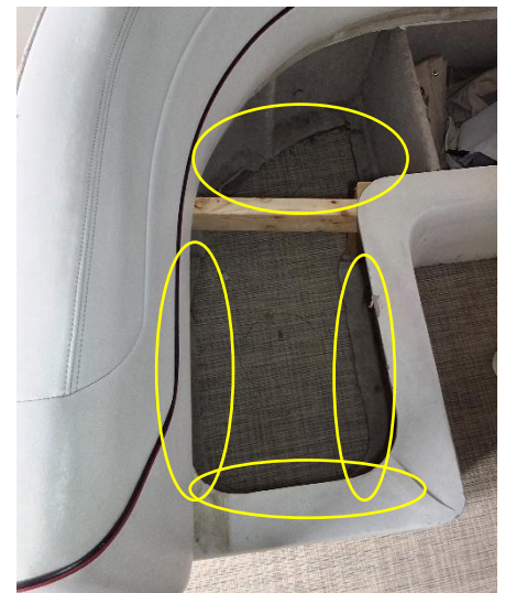
Picture 12: Port side flybridge seating with rotting plywood base.
