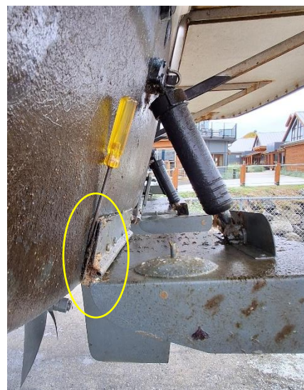
Picture 29: Port side trim tabs partially separating at the hinge.
